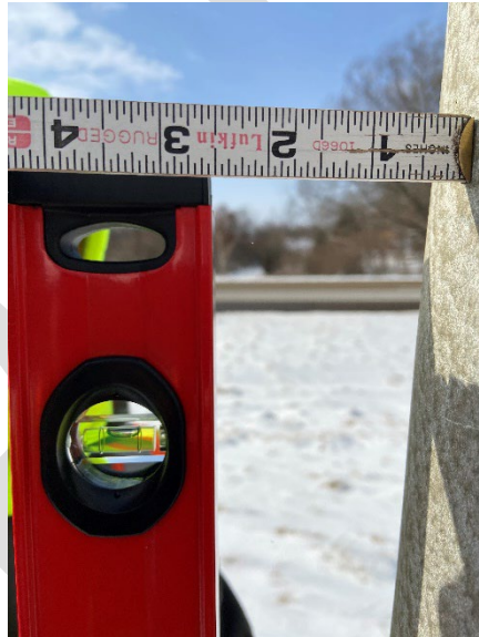
Figure 11-20: Non-frangible pole structure vertical support column (upright), visual identification of out of plumb pole (left), measurement of pole plumbness (right)
